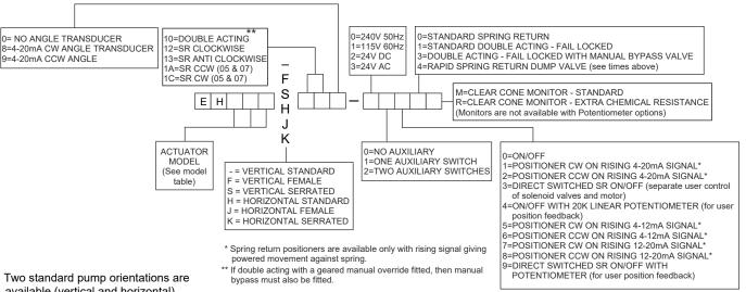
available (vertical and horizontal). Consult Kinetrol if other arrangements are required. All units will be supplied with vertical axis actuators unless otherwise specified.
