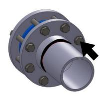
7. Centre the valve and tighten it lightly using four bolts. Add the remaining bolts (tighten them in a "criss-cross pattern").
